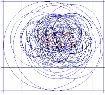
Figure 5. Deployment B. Black circles indicate ideal thresholds. Blue circles indicate required maximum measured thresholds. Black boundary indicates ideal secure area ( $339.34m^2$ ). Blue boundary indicates required secure area ( $788m^2$ ).
